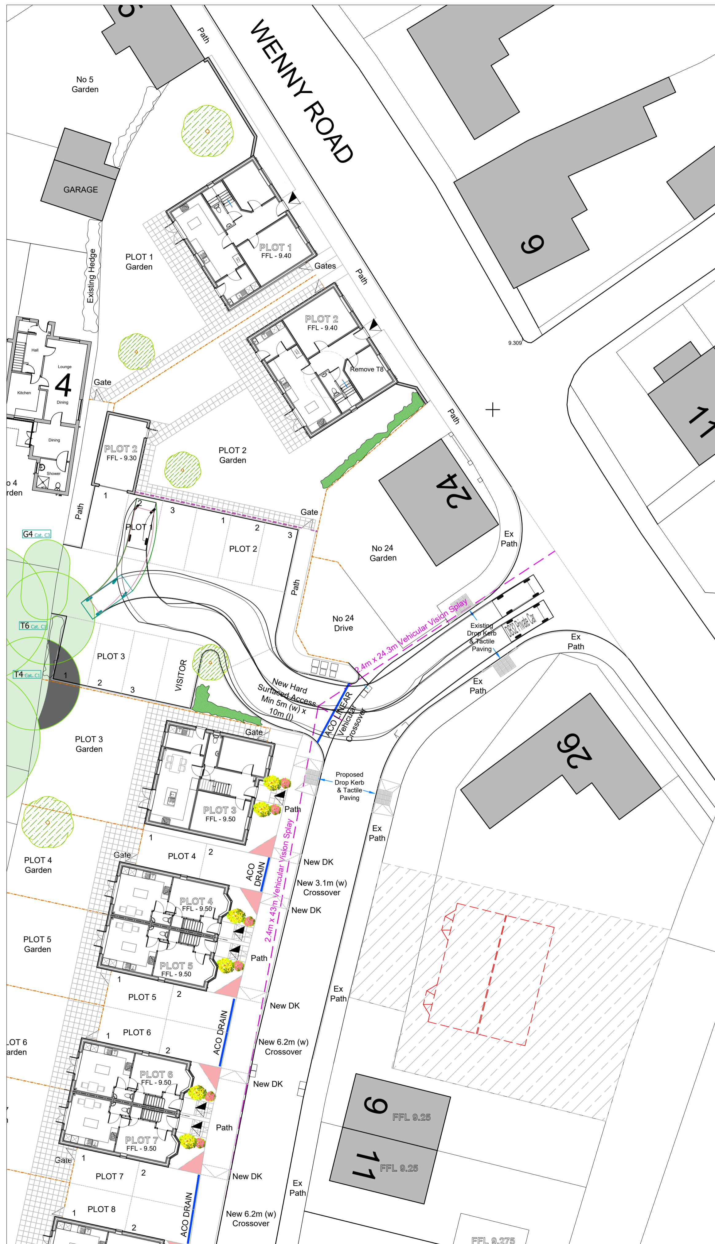
Proposed Part Site Plan (Front of Site) Showing Access for PLOTS 1, 2 & 3 Scale 1:200
